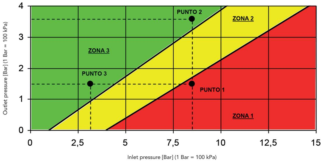
In order to avoid cavitation phenomena and therefore excessive component noise, we recommend choosing the number of pressure reducing valves necessary for a determinate pressure differential, according to the information in the "CAVITATION DIAGRAM".
