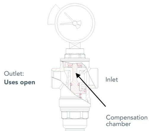
When the uses to be served are closed, the downstream pressure increases, pushing the reducer piston downwards. In this way, the shutter closes the passage section of the reducer maintaining the setting value set on the spring constant; in fact, the minimum pressure difference across the shutter permits the perfect closing of this latter.
