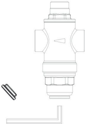
The final calibration of the pressure reducing valve must be performed with the hydraulic circuit completely full and with all the uses closed, otherwise false values would be obtained owing to the fact that the downstream pressure reduces in relation to the necessary flow rate, during any supply.
